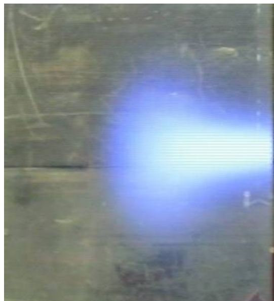
Figure 5: Imaging Bicron 400 scintillator luminescence, with the imager placed at right angles to the beam, entering the scintillator block from the right side.
